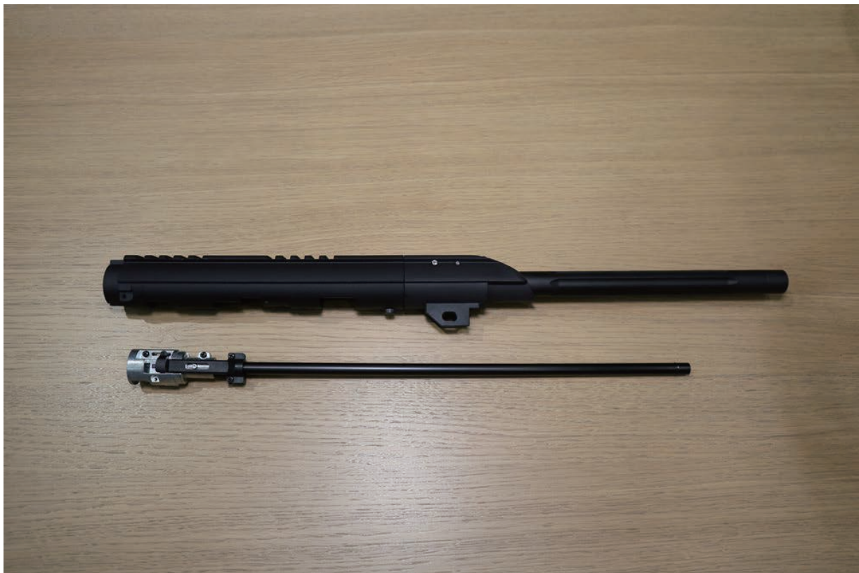
▲ Mid-receiver; 6.03mmx363mm inner barrel; metal hop-up chamber shown.
